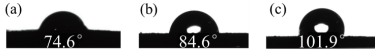
图 9 纯煤接触角测试结果(a)纯煤、(b)纯煤+柴油、(c)纯煤+ST-柴油微乳液 Fig. 9 Contact angle test results of pure coal (a) pure coal, (b) pure coal + diesel oil, (c) pure coal + ST microemulsion
