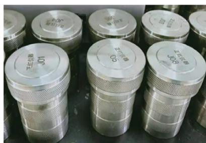
Digestion tank (adding 2mL HNO 3 +2mL HF)
