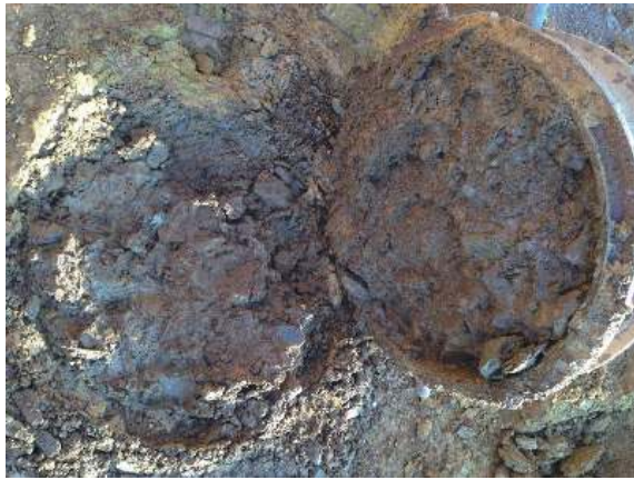
图 13 单环剪切仪得到的典型剪切破坏面 Fig. 13 Shear failure interface attained through the single box apparatus
