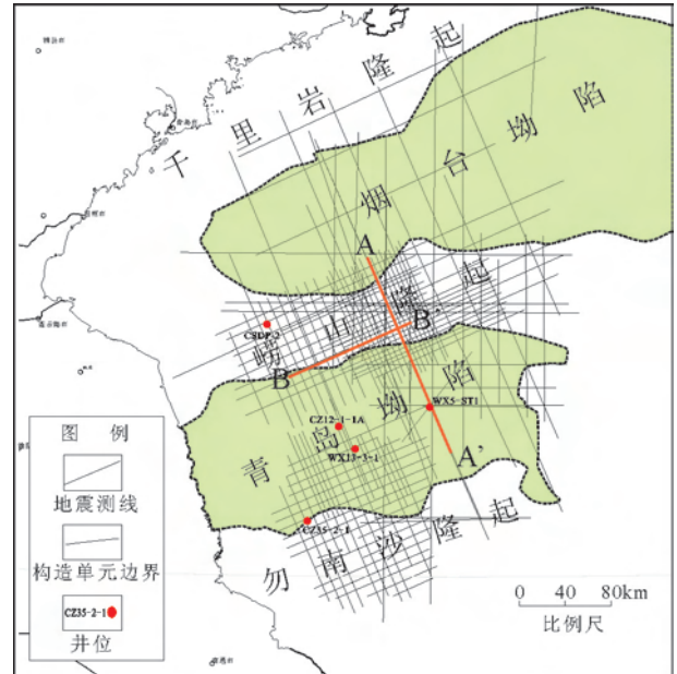
图 1 南黄海构造单元划分及地震测线、二叠系钻井分布图 Fig.1 Tectonic map of the South Yellow Sea drilling and distribution of drilling sites and seismic profiles
