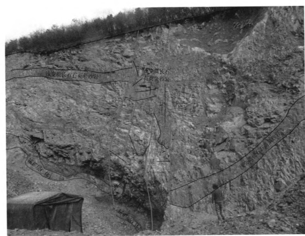
图8 茶潦矿区锰矿层及标志岩层被后期断层错断 Fig. 8 The manganese ore-body and marked stratum of Chaliao manganese deposit destructed by the faults formed later
