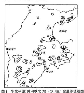
Fig. 1 NH<sub>4</sub><sup>+</sup> concentration contour of groundwater in Northern
