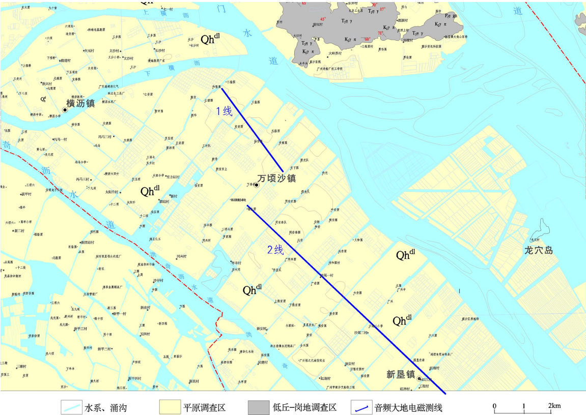
图2 研究区AMT测线布置图 Fig. 2 Layout of survey line of audio magnetotelluric in study area
