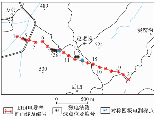
图 3 赵老园村 EH4 和对称四极激发极化法点位布置图 Fig.3 Point distribution map of the EH4 and symmetric quadrupole induced polarization in the Zhaolaoyuan village
