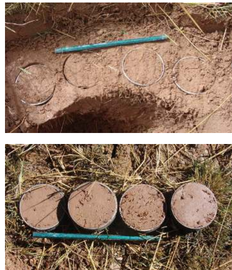
图 2 试验区 3 种草本植物根-土复合体试样原位制样过程 Fig. 2 In situ sample preparation process of the root-soil complex samples of three herbaceous plants in the testing area
