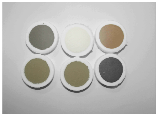
图1 经超高压压片可用于XRF或LA-ICP-MS的植物样片 Fig. 1 The plant sample pellets pretreated by high pressure compression for XRF or LA-ICP-MS analysis
