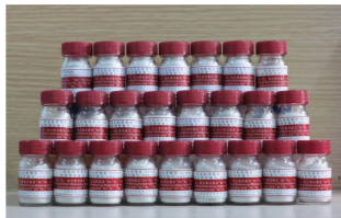
Each of the three CRMs has six property values, which are Rb, Sr, Sm, Nd concentration, 87 Sr/ 86 Sr and 143 Nd/ 144 Nd
