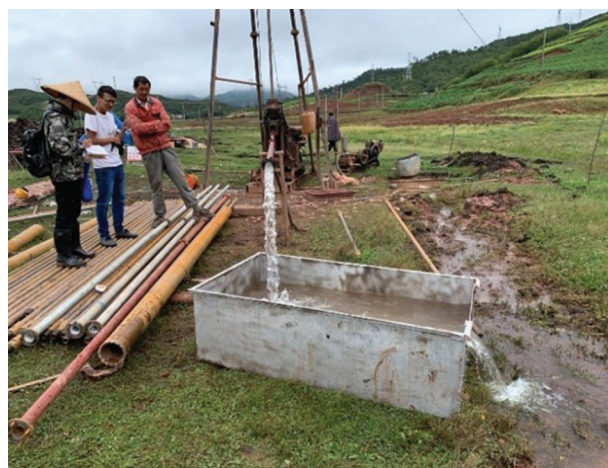
图8 昭觉县ZK01钻孔抽水试验 Fig.8 Pumping test of ZK01 drilling in Zhaojue County
