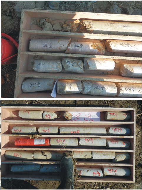
图 5 钻孔岩芯 Fig. 5 Picture of drill cores
